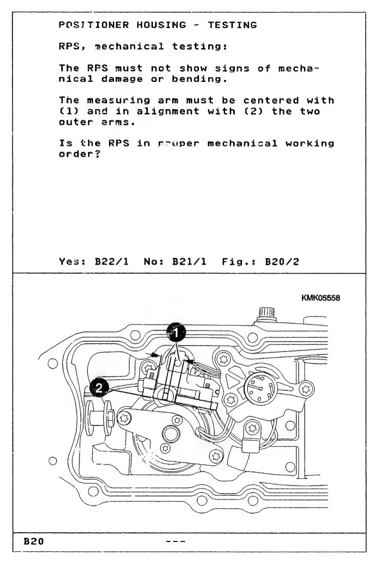
POSITIONER HOUSING - TESTING Replace damaged RPS. Pay attention to removal and installation instructions as of Coordinate: C05/1
